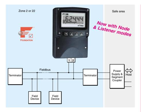
The BA444NDF-F FOUNDATION™ fieldbus Indicator is a Type n instrument that can display up to eight fieldbus process variables within a Zone 2 or 22 hazardous area. A numeric annunciator on the left hand side of the screen shows which variable is being displayed. This version of the instrument supports FOUNDATION™ fieldbus protocol; for PROFIBUS PA systems an alternative version is available – please see the BA444NDF-P PROFIBUS datasheet.
